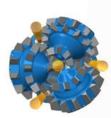
The advanced flushing system extended by additional nozzles in relation to the 3-jet flushing system system allows for more effective cleaning of the cutting structure and the bottom of the hole, and thus maintaining high drilling progress.
