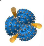
The arrangement of the nozzles and the direction of the flushing outflow allows for effective cleaning of the drill cutting structure and the bottom of the hole. This solution is designed to achieve maximum drilling progress.
