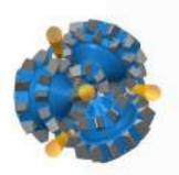
The advanced flushing system extended by additional nozzles in relation to the 3-jet flushing system allows for more effective cleaning of the cutting structure and the bottom of the hole, and thus maintaining high drilling progress.
