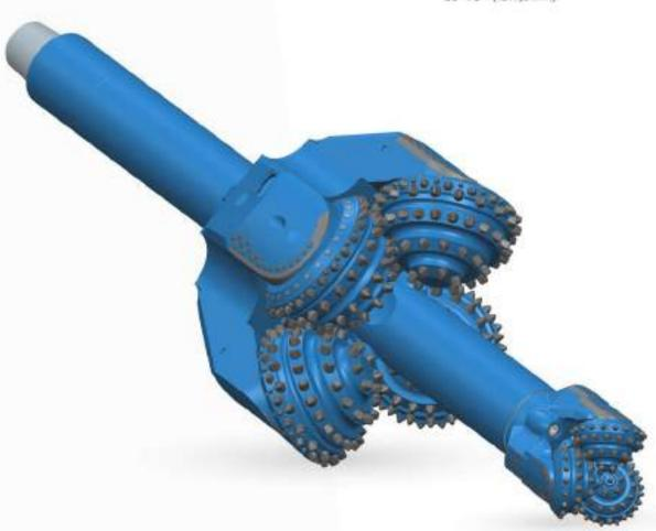
The hydraulic nozzle system provides very efficient flushing of the surface to be drilled as well as the hole opener cones. Interchangeable cone assemblies are also available for all dimensions and types of hole openers. Hole openers for hydrogeological applications can be equipped with a dedicated roller cone drill bit as a pilot.
