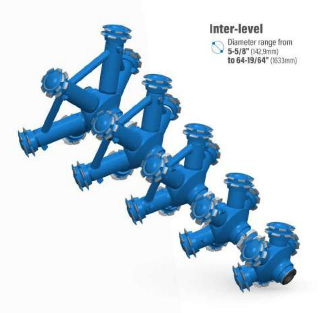
Hole openers used in mines where drilling can be carried out with a single hole opener or a set of several, interconnected hole openers system. The body is supplied with threaded connections enabling the assembly of further openers and a drilling string. These connectors are typical threaded connections used in drilling. Custom threaded connections are available based on client's requirement. Hole openers sets can be used as an alternative for riseboring applications.
