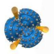
The arrangement of the nozzles and the direction of the flushing outflow allows for effective cleaning of the drill cutting structure and the bottom of the hole. This solution is designed to achieve maximum drilling progress.
